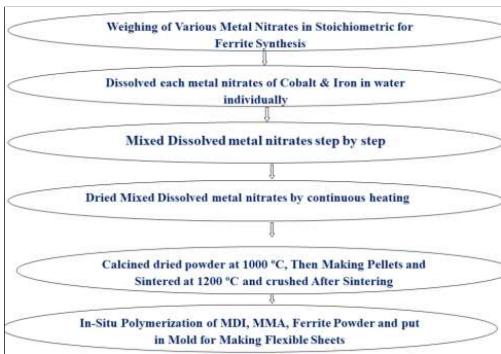
Fig 1: Step by Step Representation of Making of Flexible Mats of PU/PS IPN-CoFe 2 O 4
