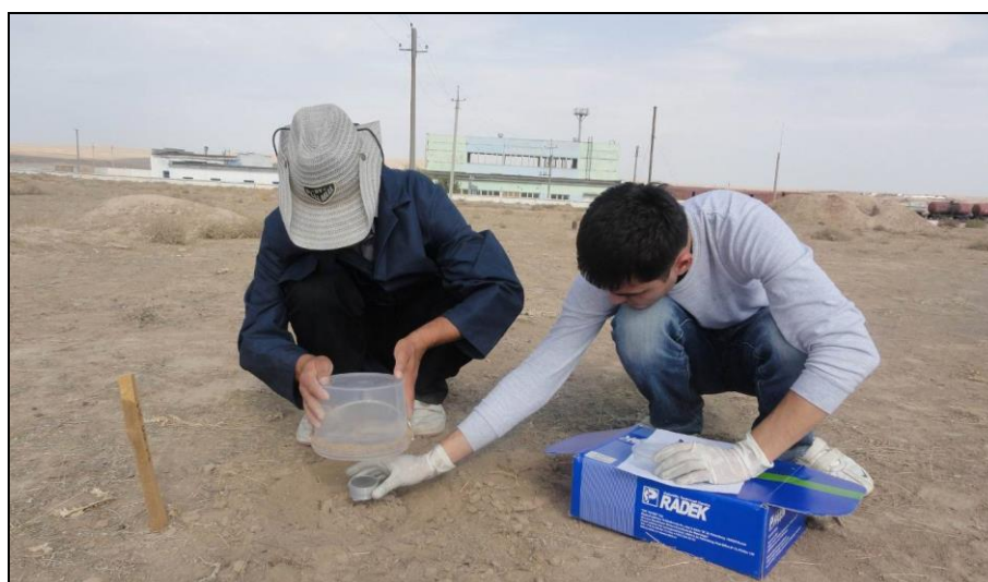
Fig 2: Sorption chamber setup.
