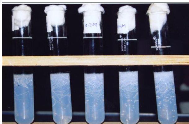
Fig 2: Growth of strontium iodate crystals
